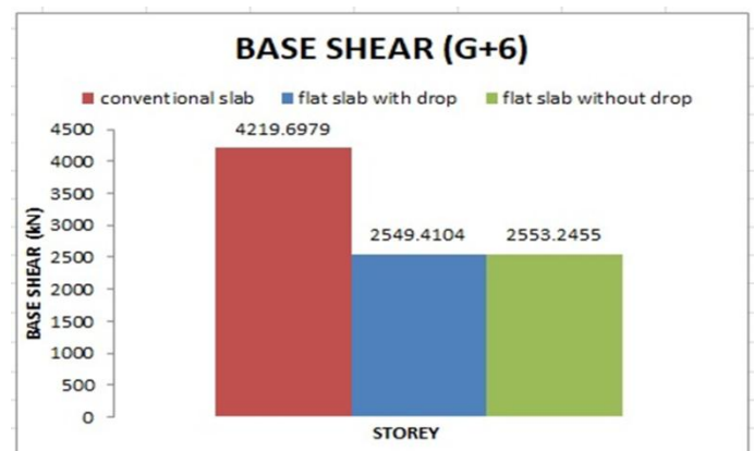
Figure-27: Base shear of G+6 building
