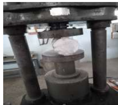
Fig.2: Split Tensile Test
