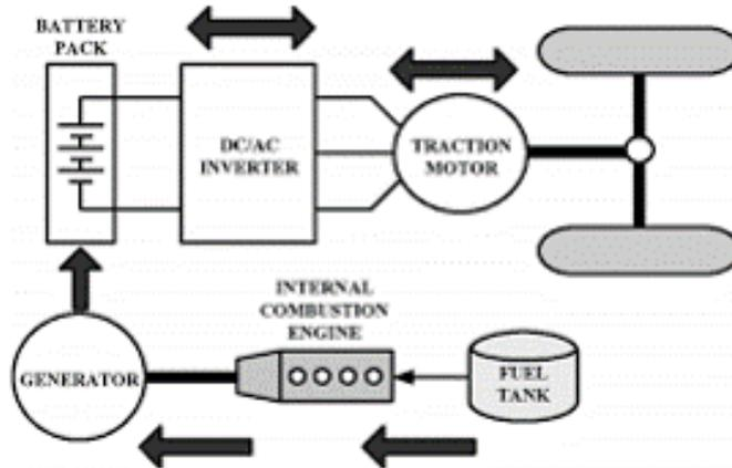
**Fig-2: Series hybrid vehicle mechanism**
