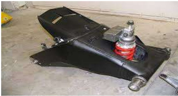
Figure (8) swing arm with mono spring coil over damper.
