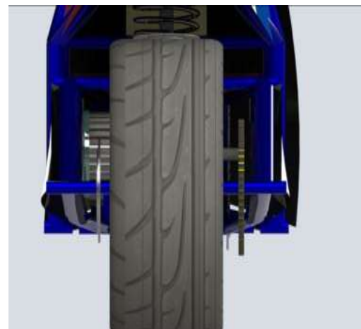
Figure (20) wet type tyre rear wheel
