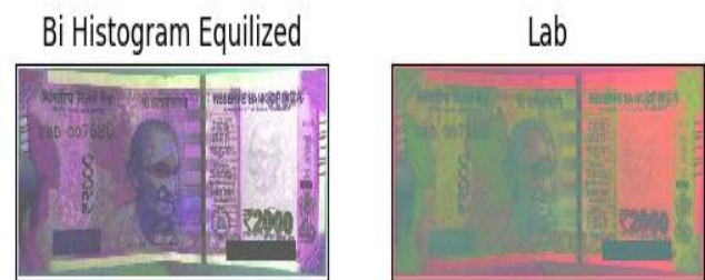
Figure 8: Brightness Preserving Bi-Histogram Equalization
