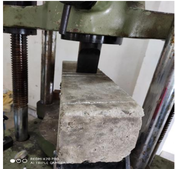
Fig. 3 Test on RCC plain beam
