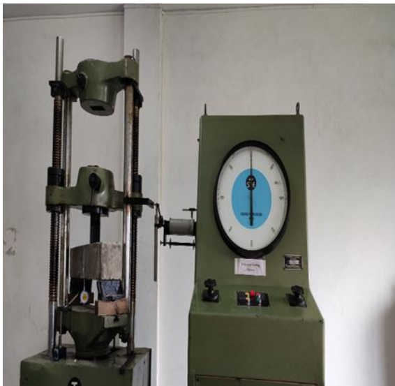
Fig. 2 Universal Testing Machine - test setup
