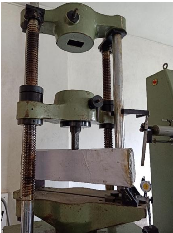
Fig. 4 Test on RCC beam with steel weld mesh and PVC flex banner
