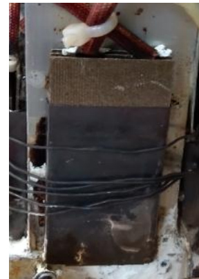
Fig -3: Heating Element
