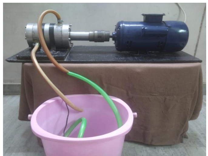
Fig-5: Fabricated Model of a Working Portable Cavitation Water Heater
