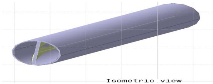
Fig 1. Views of Twisted Tube Insert
