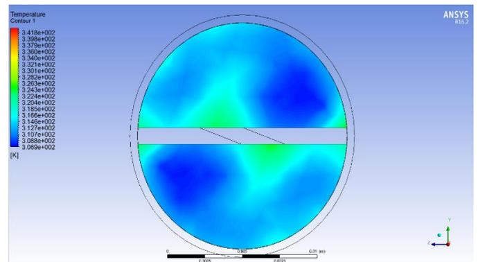
Fig 4. Outlet temperature distribution of Twisted tube at 1.2m/s velocity
