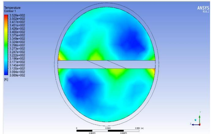
Fig 3. Outlet temperature distribution of Twisted tube at 0.1 m/s velocity
