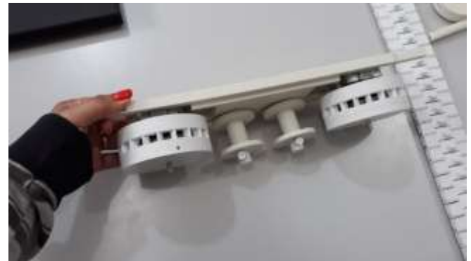
Figure 9 - Drive gears installed surrounding the engines.
