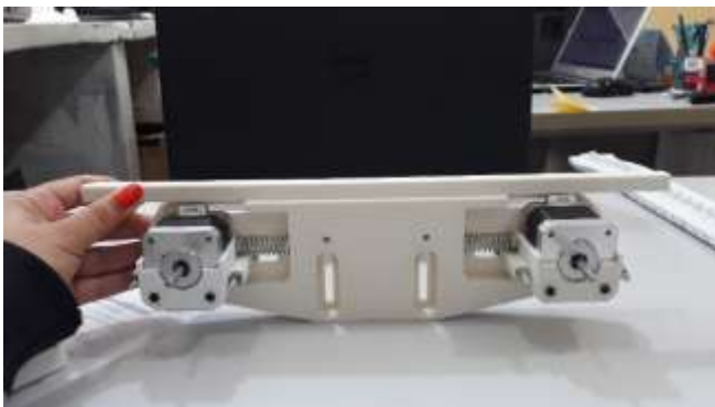
Figure 8 - Motors installed in their brackets and fixed to the side support bracket of the gears.
