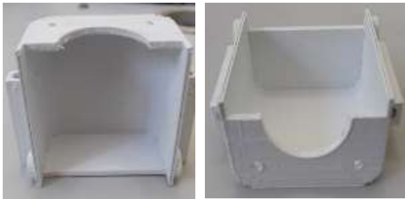
Figure 6 - Printed Propulsion Engine Support Boxes.
