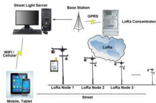
Fig-4: Street Control with IOT & LoRa Network
