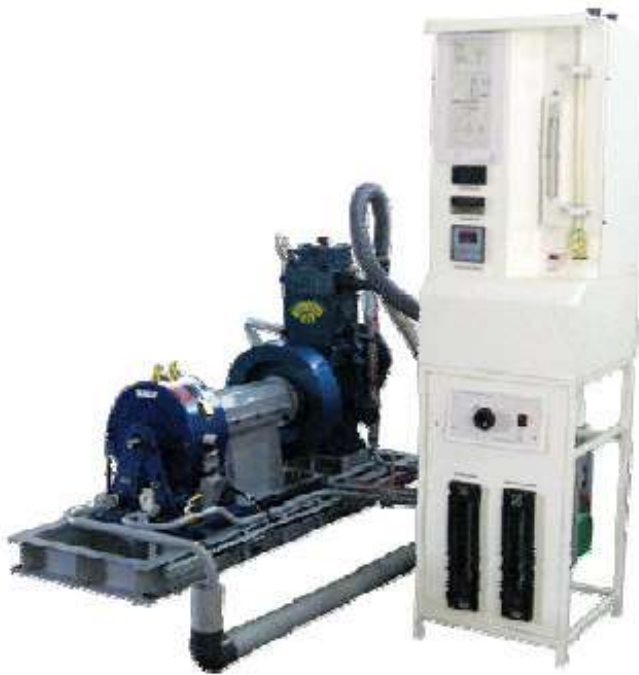
FIG.1 SINGLE CYLINDER, FOUR STROKE DIESEL ENGINE TEST RIG
