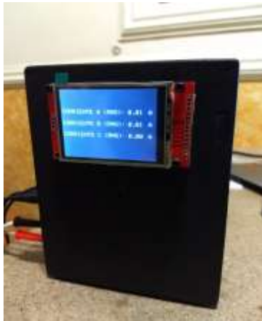
Fig. -1: Front view of the device measuring current of a three-phase motor
