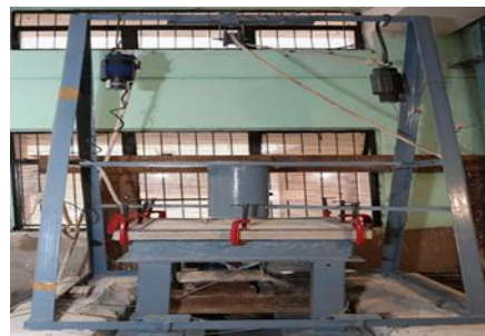
Fig.5. Impact Test Setup
