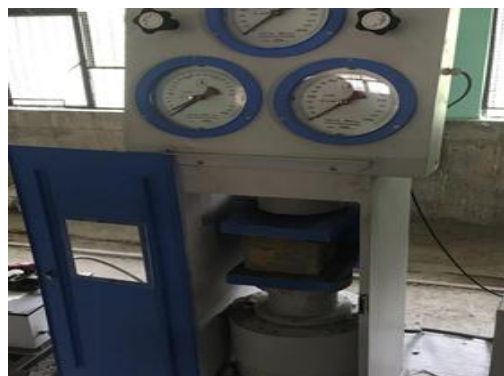
Fig.1. Compressive testing of Cubes
