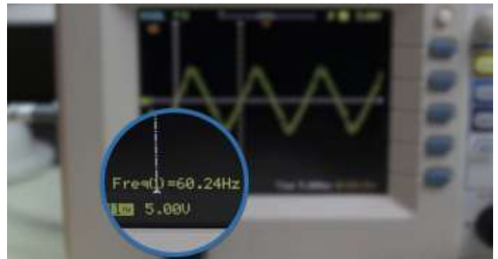
Fig -4: Frequency measurement over oscilloscope
