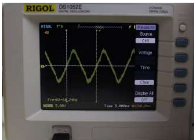
Fig -3: Signal at floating pin over oscilloscope
