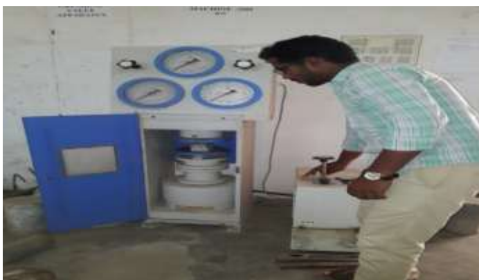
Fig: Compressive strength using UTM Machine
