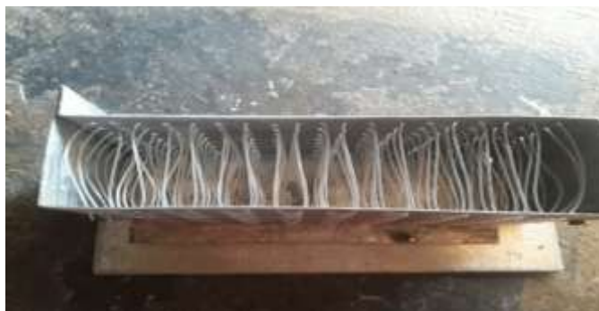
Figure: Fixing of fibers in the brick mould
