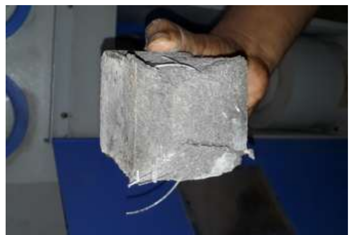
Fig: After testing on the compressive test on moulds
