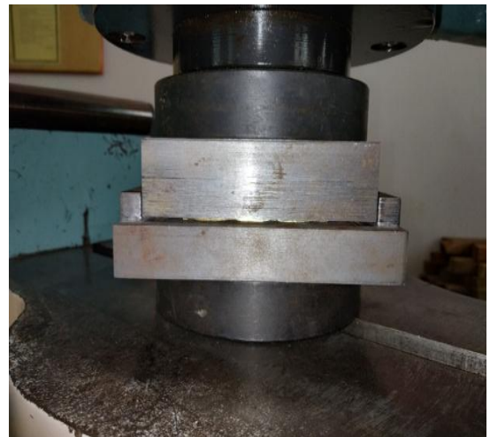
Fig 2 (b): Flattening CGP process using flat dies
