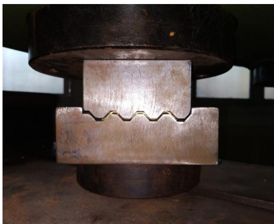
Fig 2 (a): Corrugation CGP process using flat groove corrugated dies
