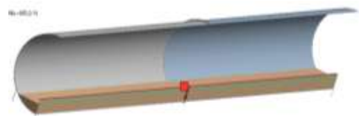
Fig -10: Load acting downwards throughout the rail
