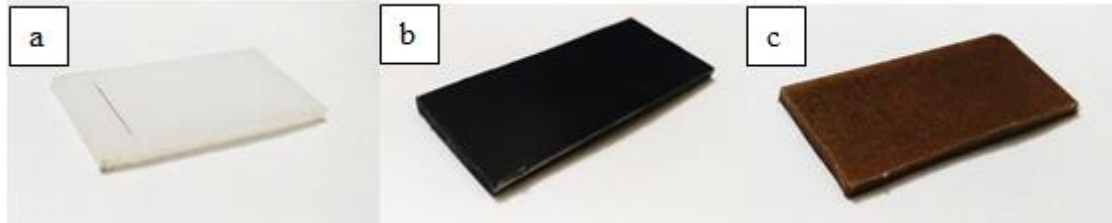
Fig -1: (a) Natural polypropylene, (b) Black polypropylene, (c) Jute fiber reinforced polypropylene
