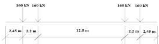
Fig-5: Standard axle distance of Nagpur metro train
