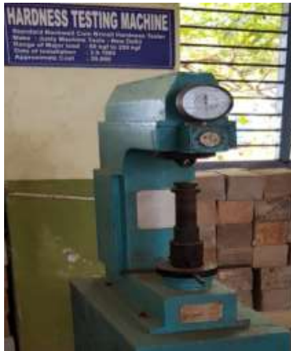
Fig 3- Brinell Harndness Testing Machine used for the experiment
