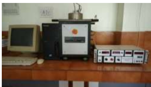
Fig 4- Pin on disc wear testing machine setup
