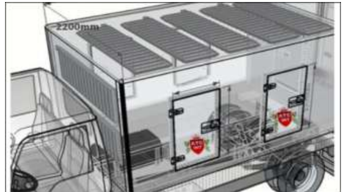
Fig - 2: PCM refrigerated truck
