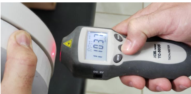
Figure 15 - Tachometer indicating the angular velocity of 110.37 rpm used in the test.
