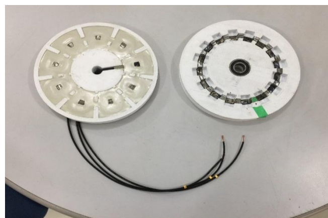
Figure 13 - Detail of the power unit.
