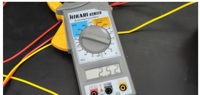
Figure 18 - Generator phase current.
