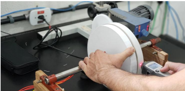
Figure 14 - Controlled bench test of the AFPM Generator.
