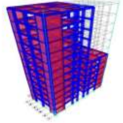
Fig 9 Model 8 Vertical Irregular Bare frame+ shear wall
