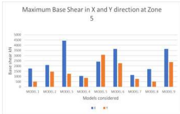
Fig 18 Graph of Maximum Base shear along X and Y direction at Zone 5
