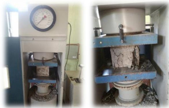
Fig 2: FAILURE OF CUBES UNDER LOADING
