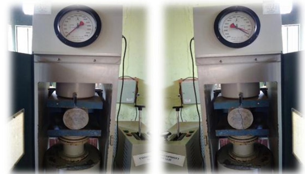
Fig 3: FAILURE OF CYLINDER UNDER LOADING
