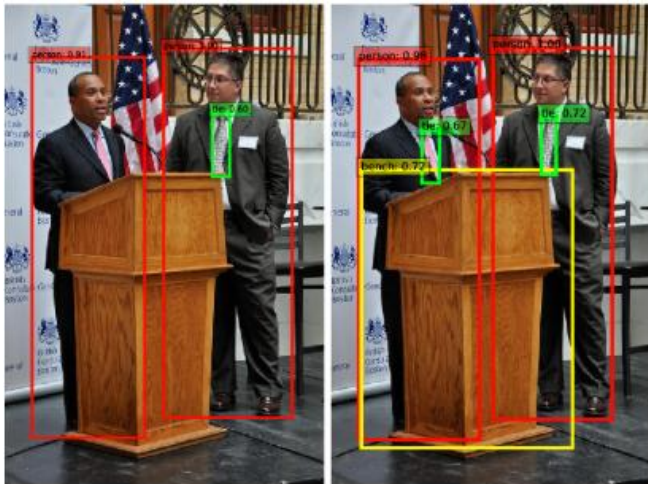
Fig.7. Example of Detections by (a) SSD and (b) DSSD showing smaller objects such as Bench and Tie detected by DSSD and neglected by SSD. Image taken from Fu et.al [18]
