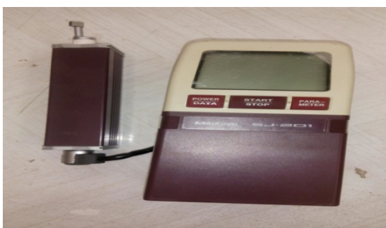
Fig - 2: Surface roughness measurement device.
