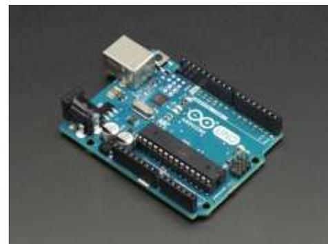
Fig 4 : Arduino Uno Board
