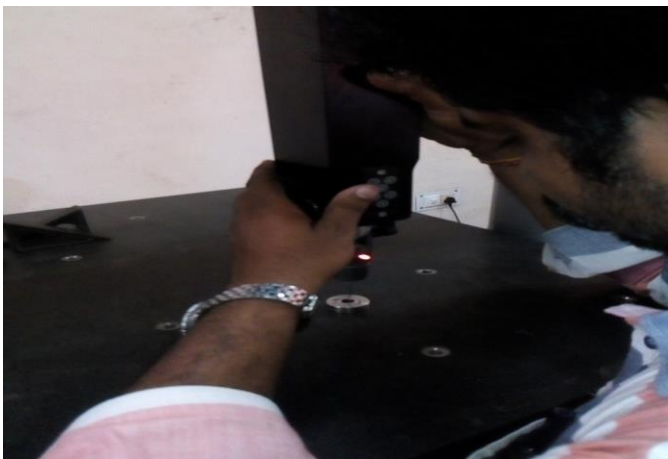
Fig 4.8 CMM Testing for Circularity Error
