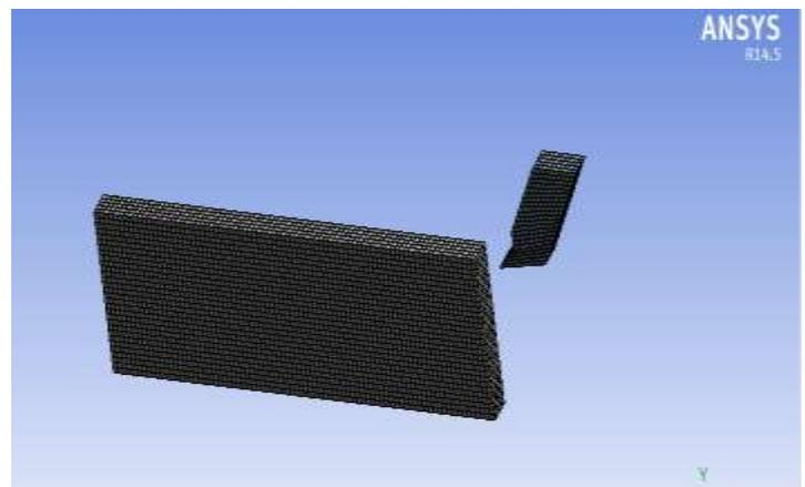
Fig 5: Meshing for work piece and tungsten tool
