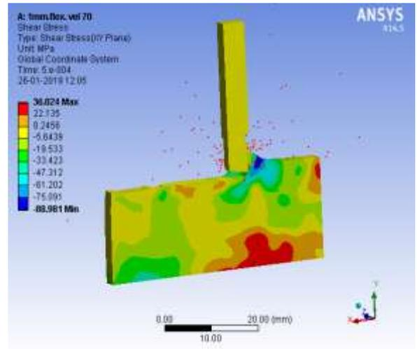
**Fig 13: shear stress at 70m/s & DOC 1mm**
