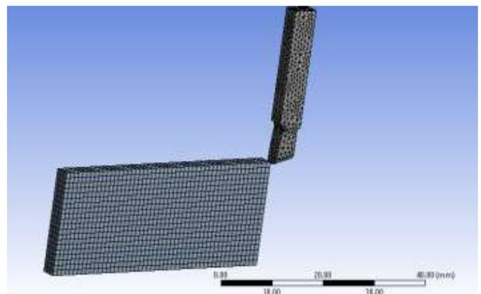
Fig 6: Meshing for work piece and steel4340 tool
