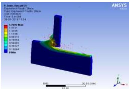
**Fig 12: Equivalent plastic strain at 70m/s & DOC 2mm**
