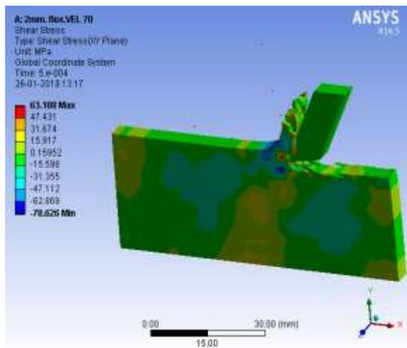
**Fig 10: shear stress at 70m/s & DOC 2mm**
