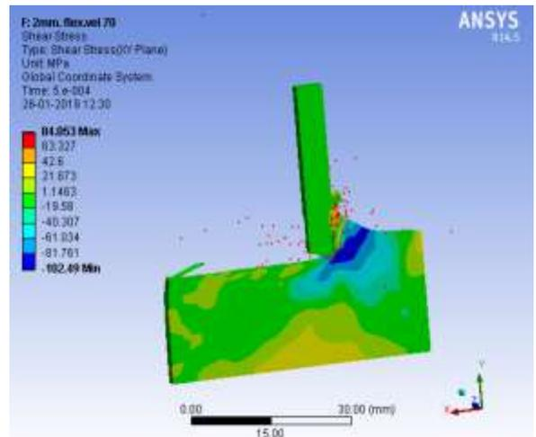
**Fig 14: shear stress at 70m/s & DOC 2mm**
