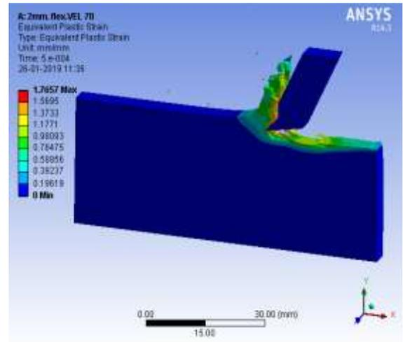
**Fig 8: Equivalent plastic strain at 70m/s & DOC 2mm**
