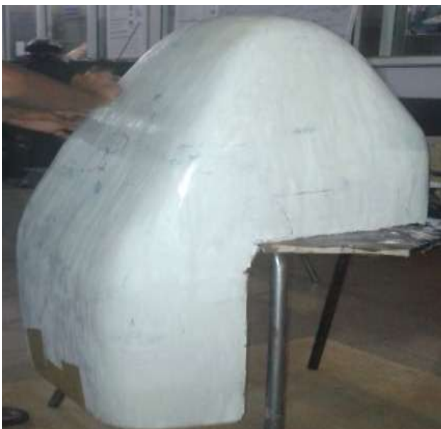
Fig -7 Finishing the surface with white plaster
