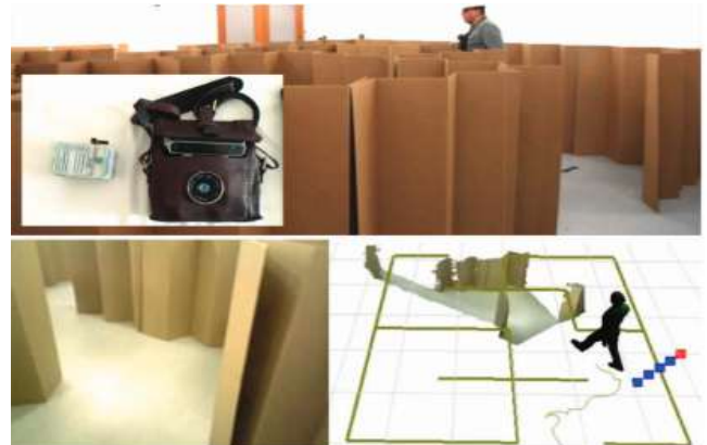
Figure 1: The wearable system enables a blind user to navigate through a maze while avoiding collisions.
