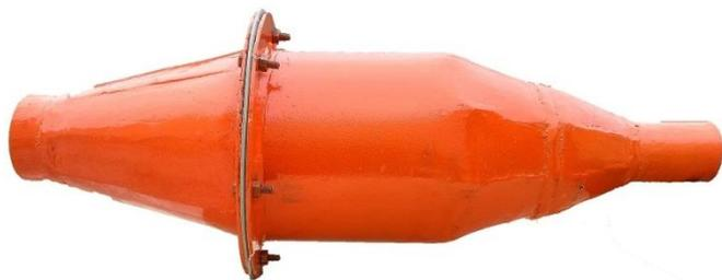
Fig -1: Fabricated Innovative Catalytic Converter
