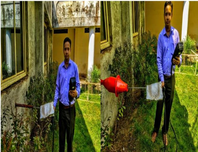
Fig -3: Emissions test before and after using Innovative Catalytic Converter using KIGAZ 310 PRO
