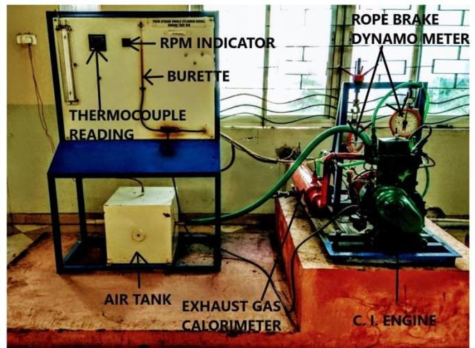
Fig -2: Four Stroke Single Cylinder C.I. engine test rig
