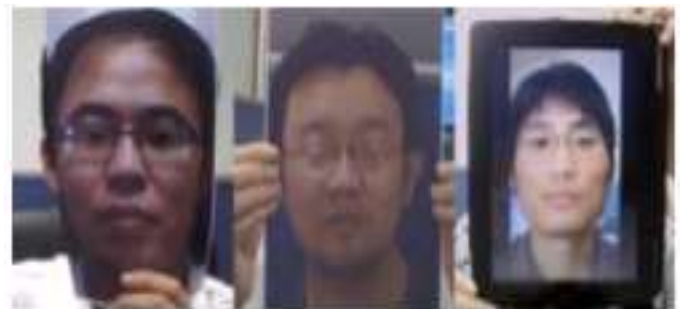
Fig: 2.3 Different fake face attacks: left, attacker hides behind the cut photo and blink; middle, another intact photo is up-down moved behind the cut one; right, is the video attack.
