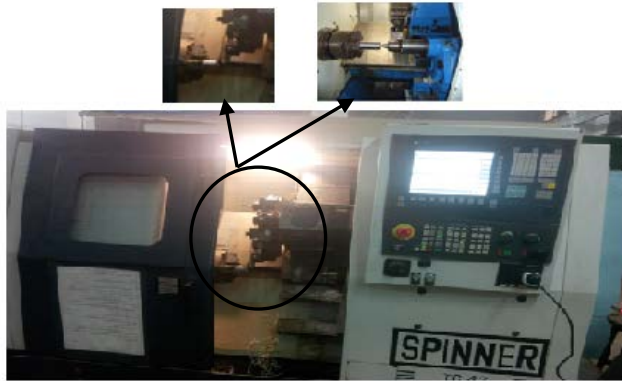
Fig - 1: CNC Lathe machine (Spinner TC42) with view of cutting zone.
