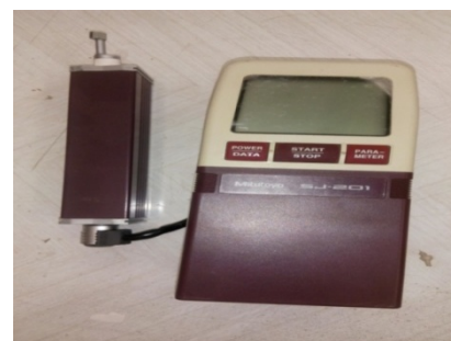
Fig - 3: Surface roughness measurement device.
