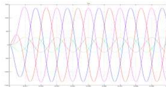
Fig 9: Three-Phase Filtered Current and Voltage
