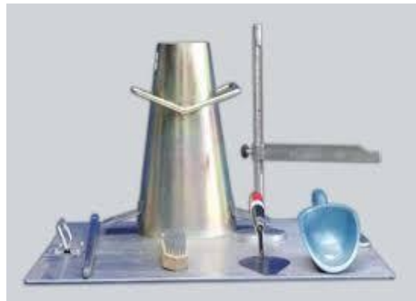
Fig-2: Slump Test equipment
