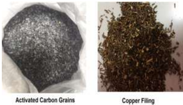
Fig. 2(c) Photograph of the used activated carbon and copper filings
