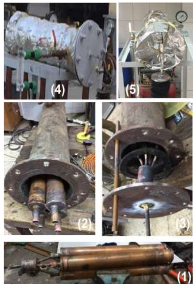
Fig. 2(b) A photographic view of the manufactured adsorbing bed and its assembling
