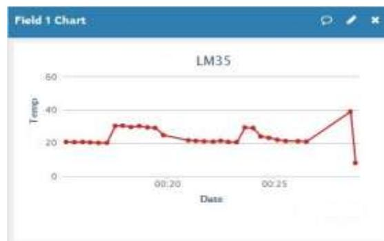
Fig-6: Temperature monitoring through IIOT
