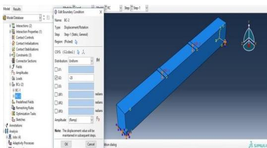
Fig - 10 : Boundary conditions in ABAQUS
