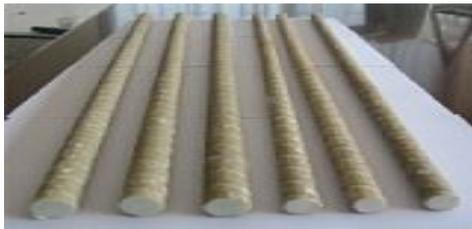
Fig - 1 GFRP Rebar
