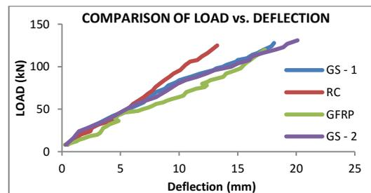
Figure.13 Plot of comparison of load vs. deflection
