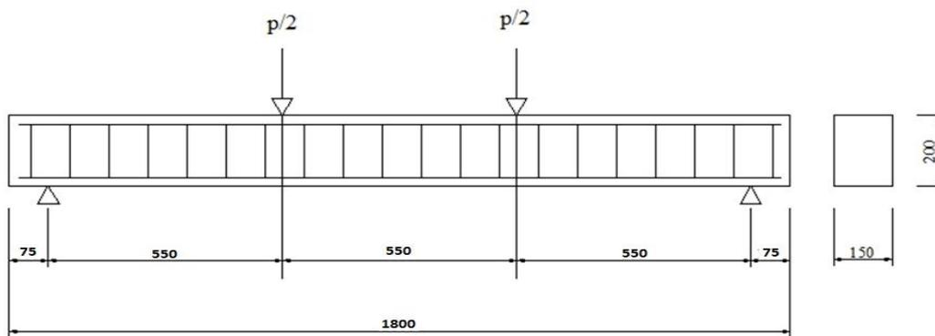
**Fig - 2 : Tested beams description—instrument and setup**
