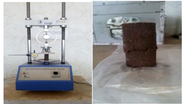
Fig -4: Testing of UCC specimen
