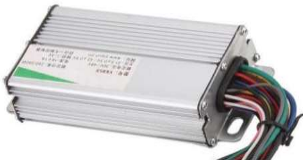
Fig -2: Motor controller for donor vehicle
