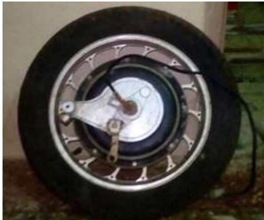
Fig -1: Hub motor with drum brake
