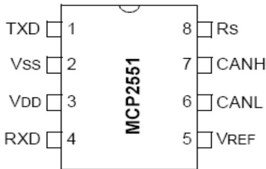
Fig2, Pin diagram of MCP2551
