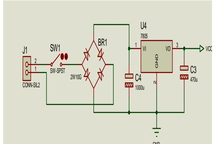
Fig3. Circuit diagram of power supply
