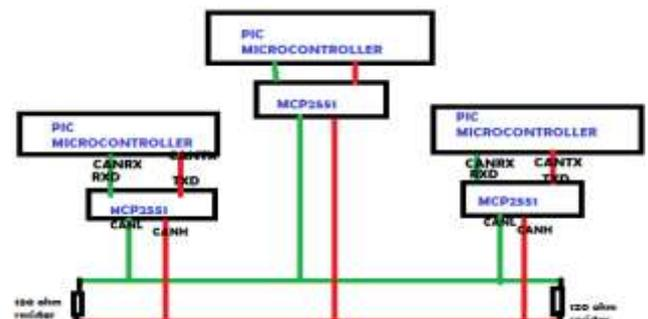
Fig4.CAN bus control area network
