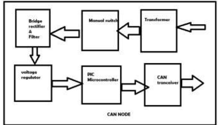
Fig5.Block Diagram of CAN node
