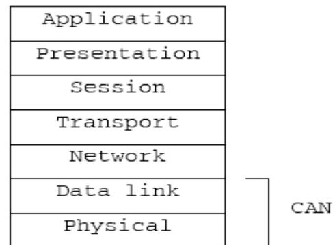
Fig.1CAN protocol defines the two layers of the OSI model.
