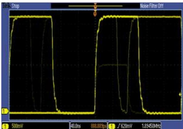
**Fig7. CAN bus signal on Tektronix Oscilloscope**
