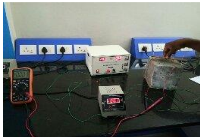
Figure2. Testing of electrical resistivity of concrete cube
