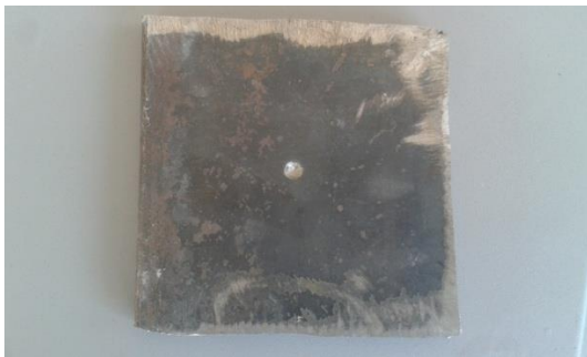
Fig 3 Mild steel model footing
