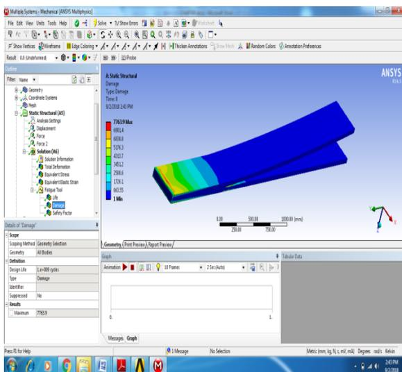
Figure 24: Damage of Aluminium alloy at X-0.7
