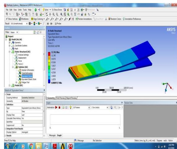
Figure 21: Stress of Aluminium alloy at X-0.7
