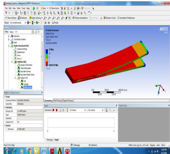
Figure 25: Safety factor of Aluminium alloy at X-0.7
