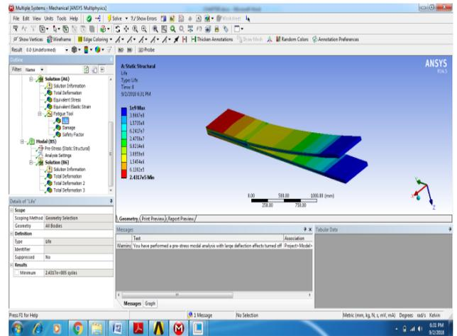
Figure 14: Life of S-2 Glass fiber reinforced polymer composite at X=0.7
