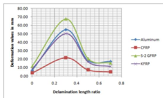
**Figure 29: deformation values of different materials v/s delamination ratios**
