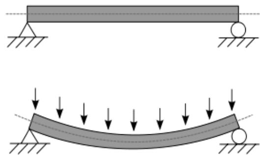
**Figure 1: A statically determinate beam, bending (sagging) under a uniformly distributed load**
