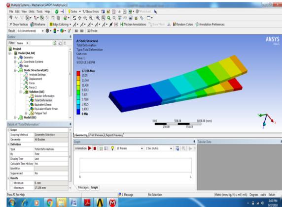
Figure 20: Total deformation of Aluminium alloy at X-0.7
