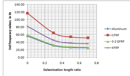
Figure 34: 3<sup>rd</sup> frequency of different materials v/s delamination ratios
