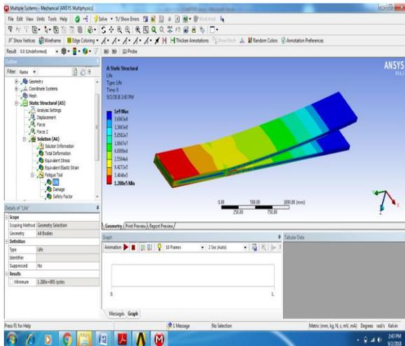
Figure 23: Life of Aluminium alloy at X-0.7
