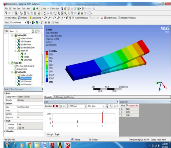
Figure 26: Total deformation 1 of Aluminium alloy at X-0.7
