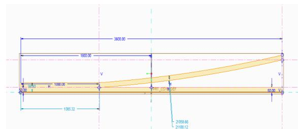
**Figure 8: 3D model of delaminated cantilever beam at X-0.7**
