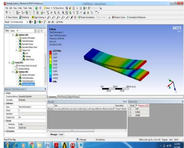
Figure 19: Total deformation 3 of S-2 Glass fiber reinforced polymer composite at X-0.7
