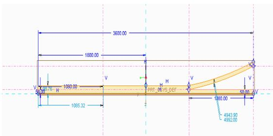
**Figure 4: 2D model of delaminated cantilever beam at X-0.3**
