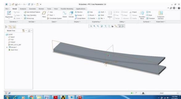
**Figure 7: 3D model of delaminated cantilever beam at X-0.7**
