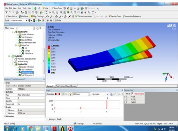
Figure 27: Total deformation 2 of Aluminium alloy at X-0.7
