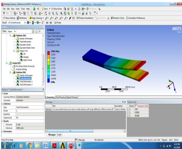
Figure 17: Total deformation 1 of S-2 Glass fiber reinforced polymer composite at X-0.7
