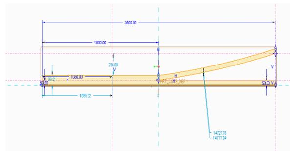
**Figure 6: 2D model of delaminated cantilever beam at X-0.5**
