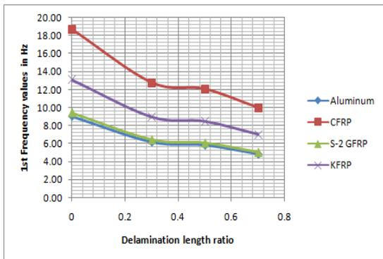
Figure 32: 1<sup>st</sup> frequency of different materials v/s delamination ratios
