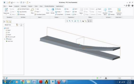
**Figure 5: 3D model of delaminated cantilever beam at X-0.5**
