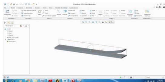
**Figure 3: 3D model of delaminated cantilever beam at X-0.3**
