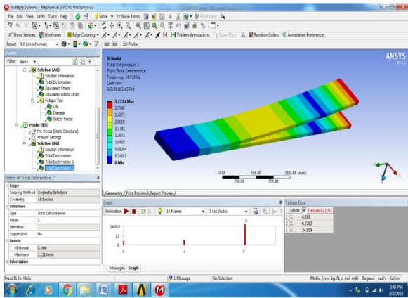
Figure 28: Total deformation 3 of Aluminium alloy at X-0.7
