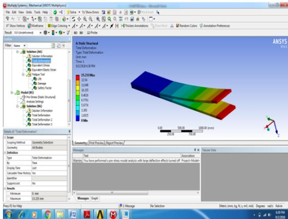
Figure 11: Total deformation of S-2 Glass fiber reinforced polymer composite at X=0.7
