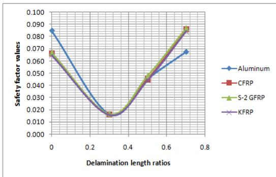
Figure 31: Safety factor of different materials v/s delamination ratios
