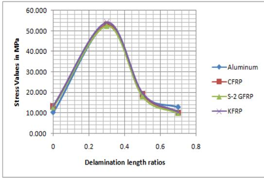
Figure 30: Stress values of different materials v/s delamination ratios
