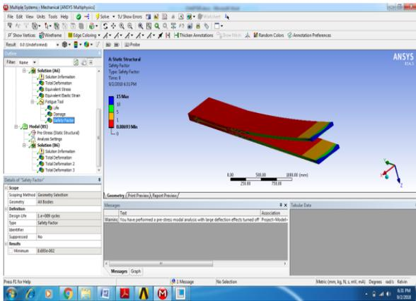
Figure 16: Safety factor of S-2 Glass fiber reinforced polymer composite at X-0.7
