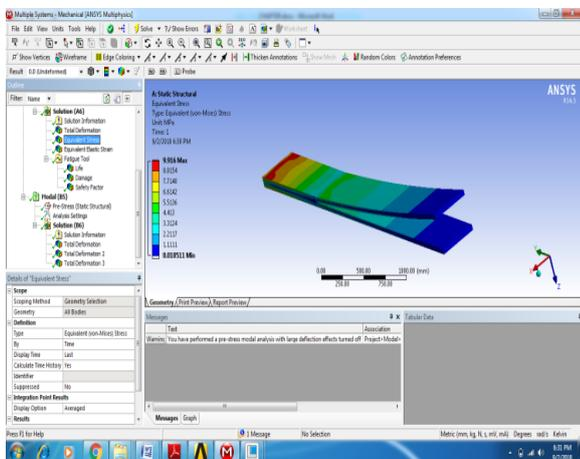
Figure 12: Stress of S-2 Glass fiber reinforced polymer composite at X=0.7
