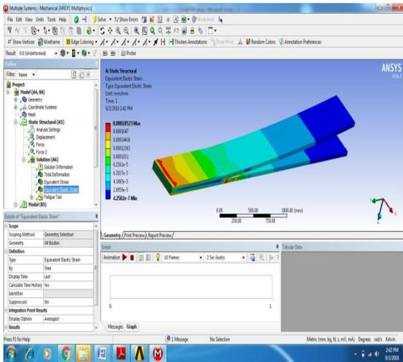
Figure 22: Strain of Aluminium alloy at X-0.7
