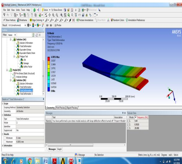
Figure 18: Total deformation 2 of S-2 Glass fiber reinforced polymer composite at X-0.7
