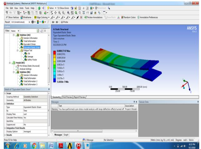
Figure 13: Strain of S-2 Glass fiber reinforced polymer composite at X=0.7
