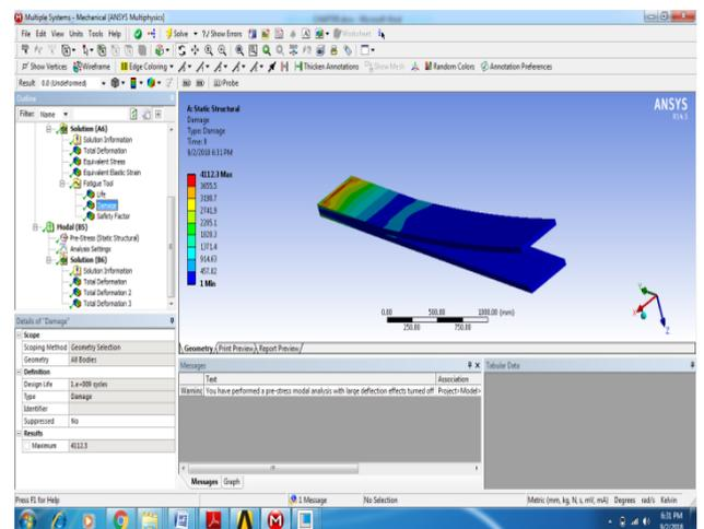
Figure 15: Damage of S-2 Glass fiber reinforced polymer composite at X=0.7
