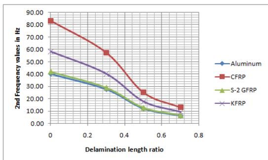
Figure 33: 2<sup>nd</sup> frequency of different materials v/s delamination ratios
