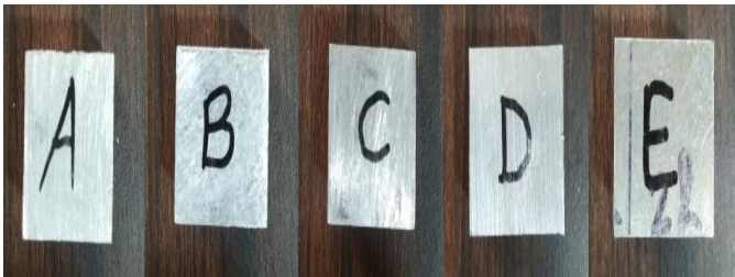
Fig -1: Sample of Aluminium Alloy Prepared by Casting and Cutting
