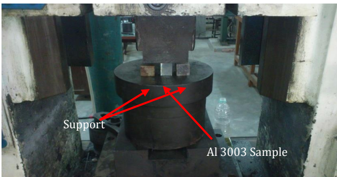
Fig -3: Forging of Sample on the Forging Machine
