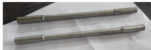
Fig. 3 mild steel specimen of 10 mm diameter
