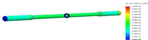
Fig.9 Stress Distribution in Butt Welded Specimen in solid works
