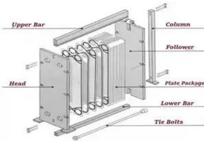
Fig.1 Exploded view of PHE
