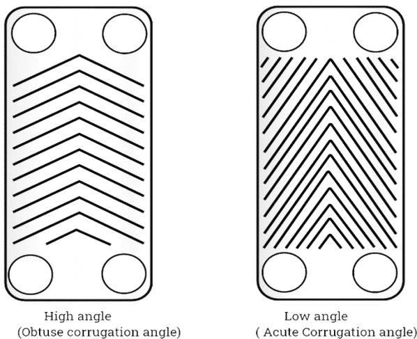
Fig.2 A typical plate of a PHE
