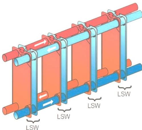
Fig.6 Semi-welded PHE
