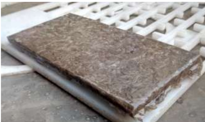
Fig -1: Prepared sheet for Jute composite
