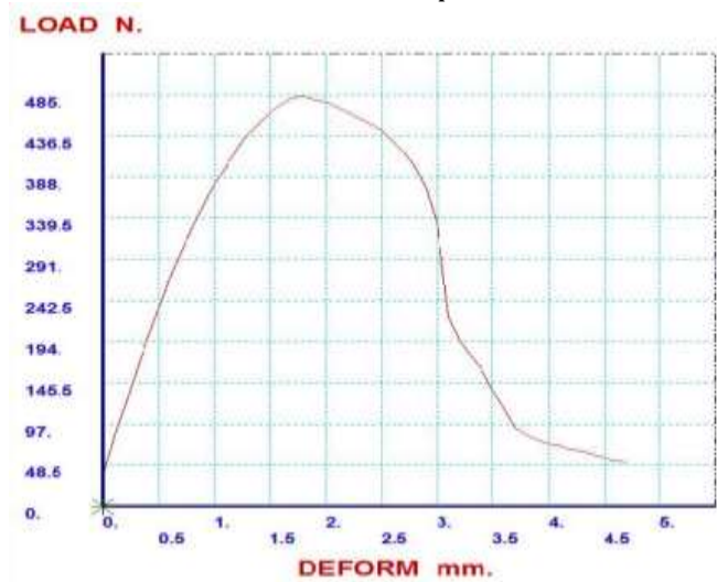
Fig 7: Load VS deformation diagram during Flexural test for Jute Composite
