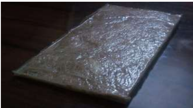
Fig -2: Prepared sheet for Banana composite
