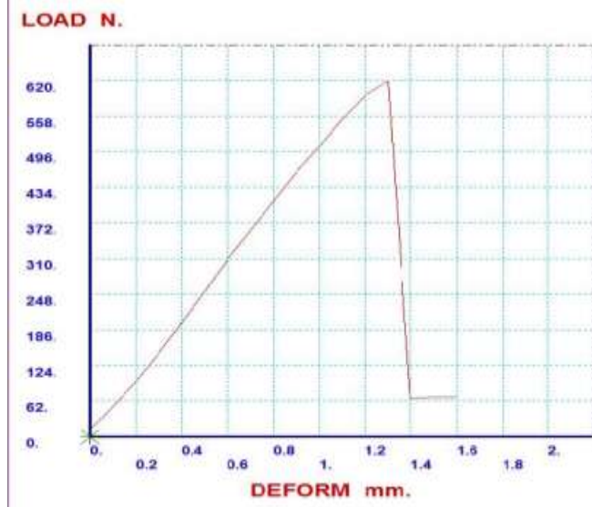
Fig 6: Load VS Deformation diagram during Flexural test for Banana Composite
