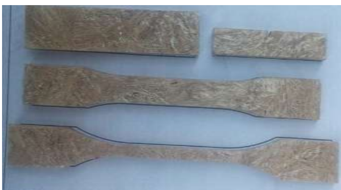
Fig -3: Specimens after Waterjet Cutting
