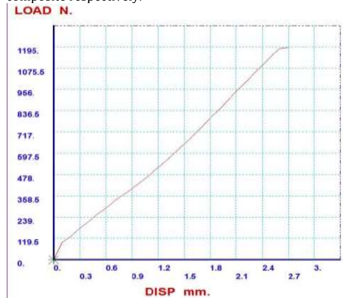
Fig -4: Load VS Displacement diagram during tensile test for Banana composite
